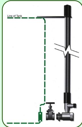
Suits Standard 1" BSP Connections. Max. Height - 1830mm
