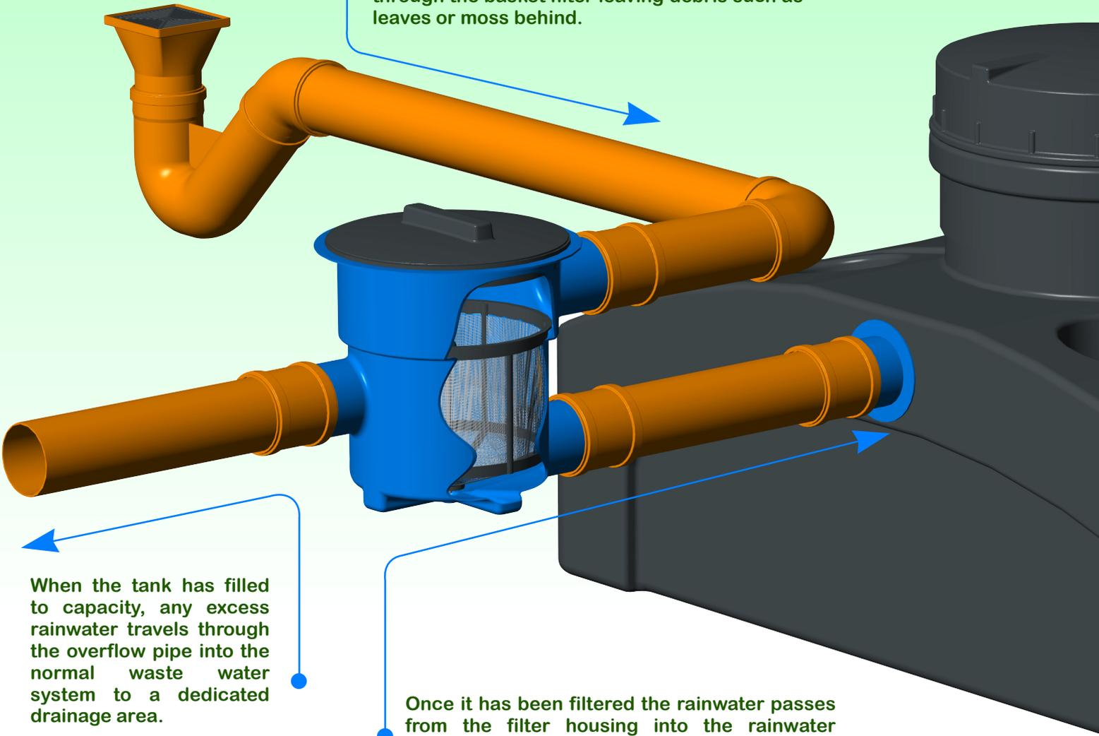
When the tank has filled to capacity, any excess rainwater travels through the overflow pipe into the normal waste water system to a dedicated drainage area.
