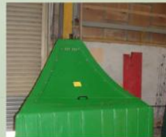
Musoir Filling hatch (for water or sand)
