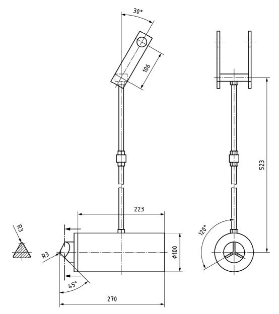
Figure C.1 — Impact test equipment
