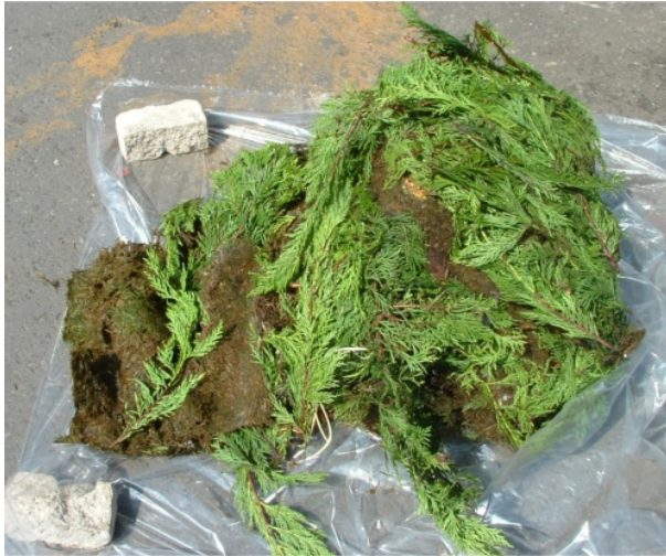
Contents of Standard 140lt Wheel Bin after three weeks. Contents were wet, loose and semi-composted.
